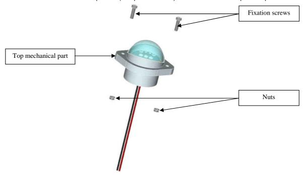
Place the equipment in its aircraft location. The equipment must be oriented as described in the picture below.
