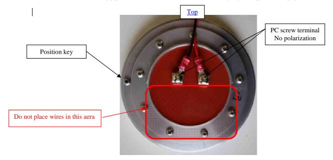
Place the equipment in the aircraft mounting part (see picture below). If available, ensure that the
